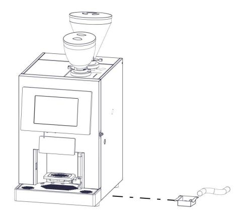
Then make a hole in the plastic drip tray (see image below). In this way the liquid collected, will be discharged externally through the tube that was previously connect ed (previous step).
