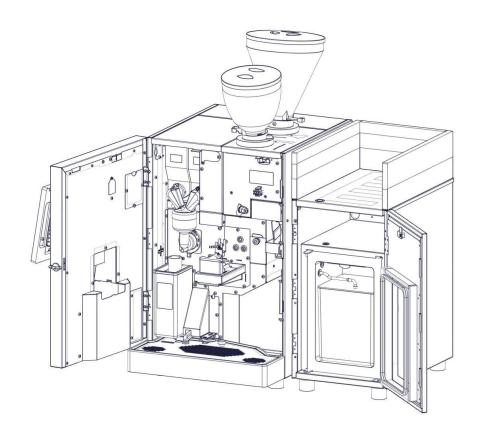
Connect the pipe to the black plug of the milk container as indicated on the image below
