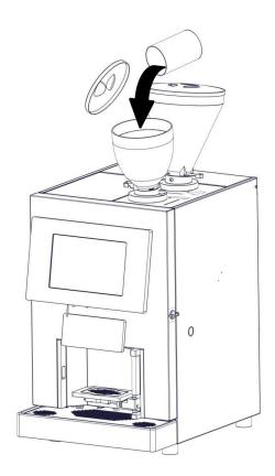
Remember to open the beans stopper located at the bottom of the coffee beans hopper. (see image A below).
