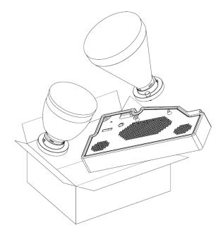
Extract the coffee hopper/s from the box and install it in the neck on the top lid of the HLF 3700R coffee machine, turn it clockwise until the micro fits into the hole (see image below).
